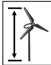
**Tower.** The monopole, guyed monopole or lattice structure that supports a wind generator.
