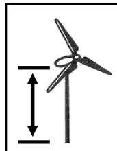
**Wind generator.** The blades and associated mechanical and electrical conversion components mounted on top of the tower whose purpose is to convert kinetic energy of the wind into rotational energy used to generate electricity.
