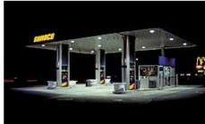
The above photographs illustrate the impact of glare on a lighting installation. The left photo has high-glare, non-recessed fixtures under the canopy. Note how bright the lights themselves are and how dark the pump area is. The right photo shows the same gas station canopy with full-cutoff, recessed fixtures. Note how the light is directed effectively toward the gas pumps. Images from <a href="http://www.skyandtelescope.com">http://www.skyandtelescope.com</a>
