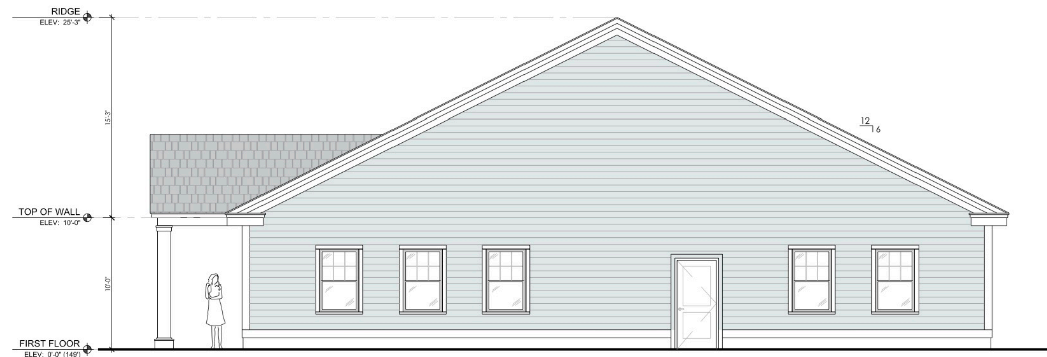
4 SIDE ELEVATION (EAST) SCALE: 1/4" = 1'-0"
